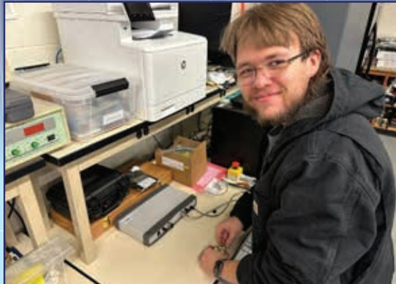
Student works on measuring the dielectric permittivity of epoxy samples with and without nano particle additives.
