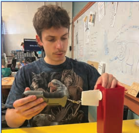
NEEC student testing a magnetically attached fin.
