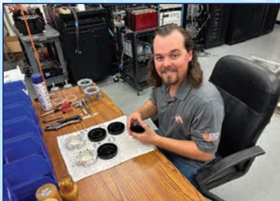
Student prepares molds for making epoxy samples with and without nano additives.
