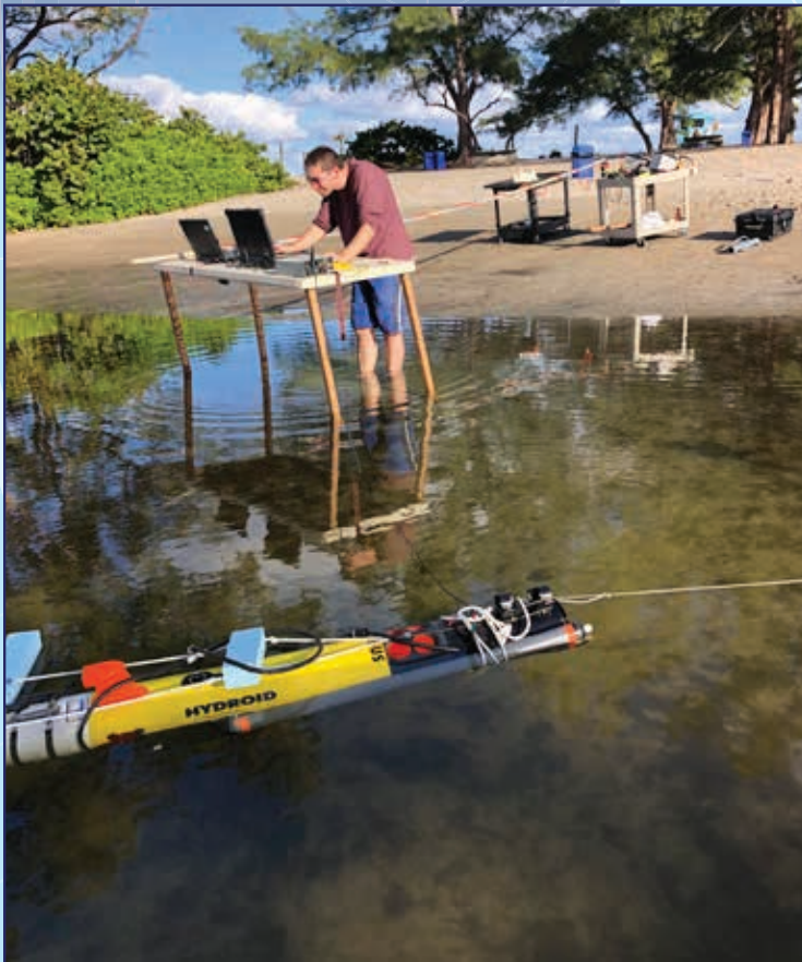
NEEC student performing field experiments with a modified REMUS 100 UUV.
