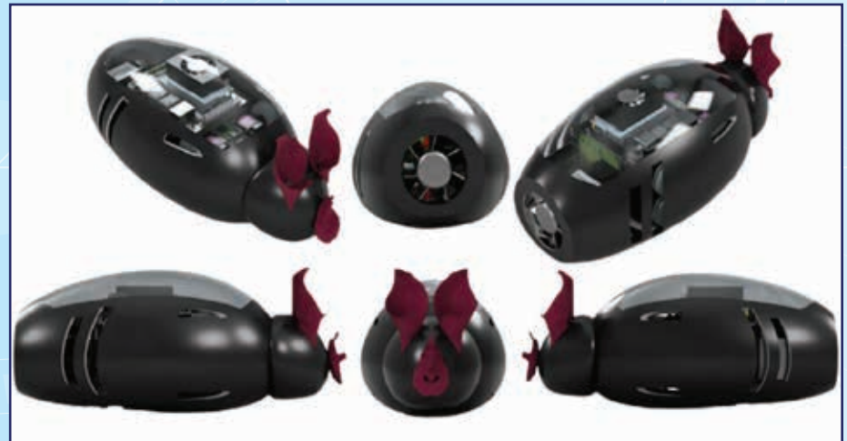
Rendering of the CAD model for the shell and interior for the next-generation prototype of the biomimetic sonar head with soft-robotic, tension-driven actuation.
