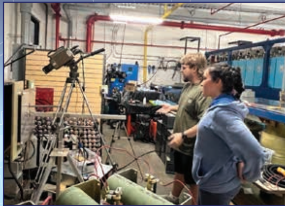
Students set up an arc flash experiment in which a high voltage electric double layer capacitor is being studied.
