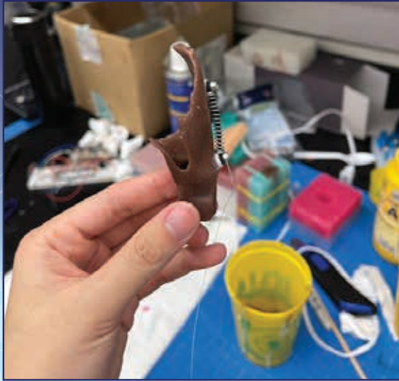
Student team working on a tension controlled biomimetic pinna actuation mechanism as their senior design capstone.
