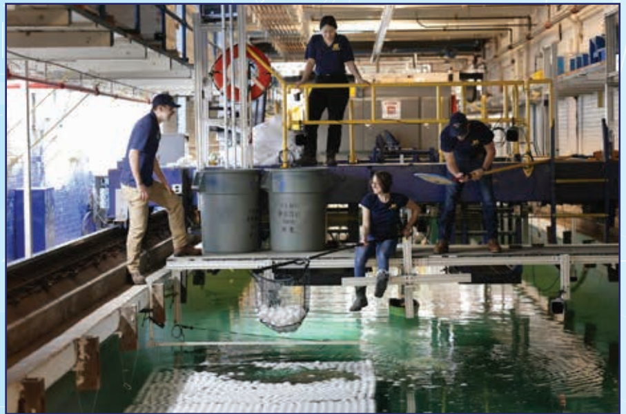
Student team on carriage of Aaron Friedman Marine Hydrodynamics Laboratory preparing ice field for a day of testing.
